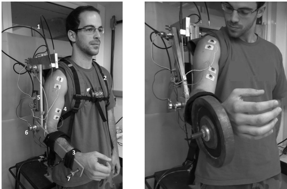
Figure 8. The exoskeleton system (left); and a trial with a 7 lb (3.2kg) payload (right)
