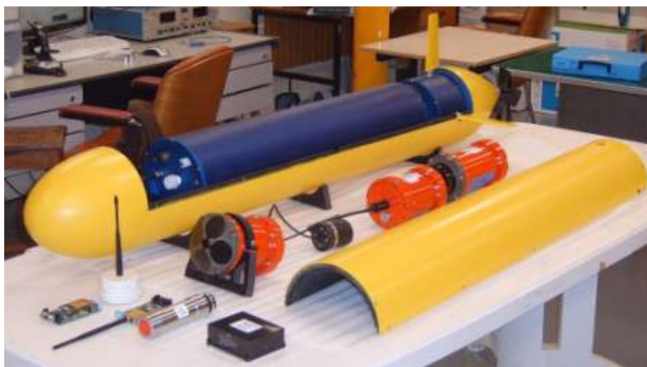
Figure 2. The Pirajuba AUV external hull, pressure vessels, external sensors and wireless communication hardware. Inside the vehicle, it is shown the maneuver and the main vessels.
