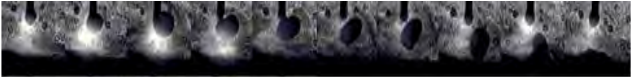
Figure 7. Globular transfer mode.
