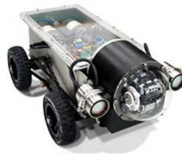
Figure 4. PIC for internal inspection (Subsin, 2010)
