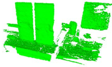
Figure 7. Reconstructed scene for a small translational (3 cm) movement of the sensor.
