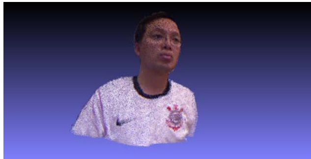
Figure 9. Point Cloud generated by the ICP for a small rotational (40 degrees) movement of the sensor.
