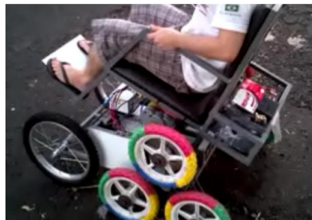
Figure 6. Chair transposing small obstacle and seat tilt test.
