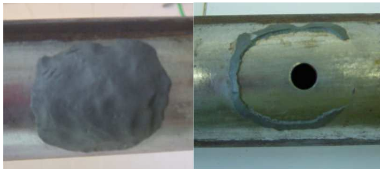
Figure 7: Epoxy Repair System A
