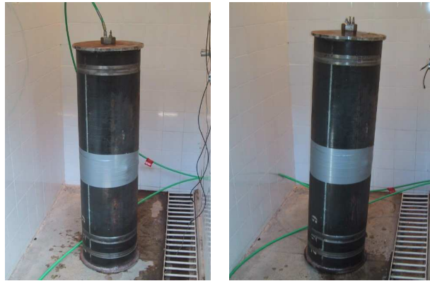
Figure 10: 12" SCH 20 steel pipe with a repair of a hole of 10mm before and after testing
