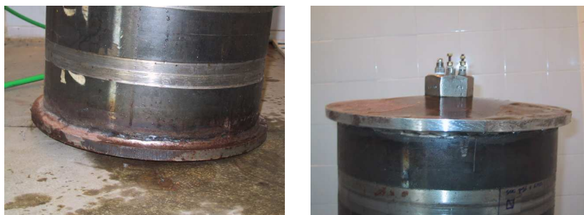
Figure 11: Deformed caps after testing at 60 \text{ kg/cm}^2 and 80^\circ\text{C} .
