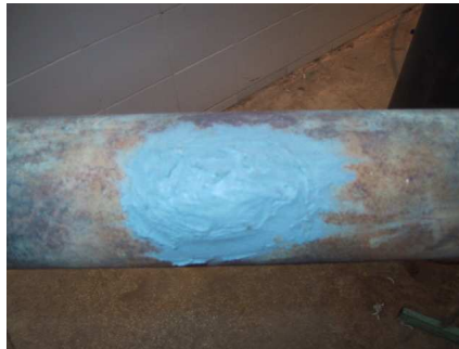
Figure 9: Epoxy Repair system C
