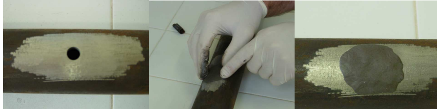
Figure 3: Epoxy repair procedure
