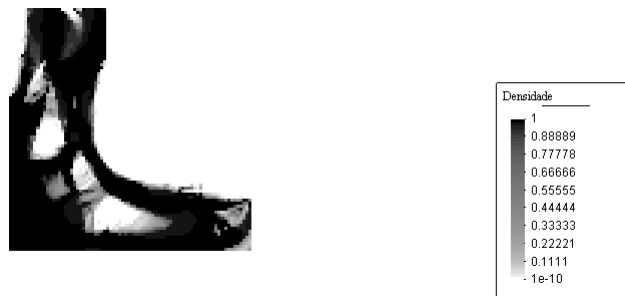
Figure 5: L-shaped domain optimal design for two load cases
