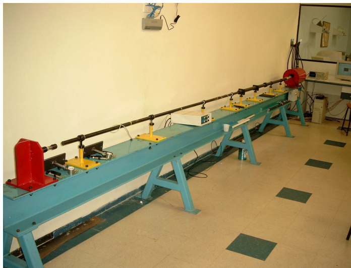
Figure 6: Hopkinson bar in GMSIE.
