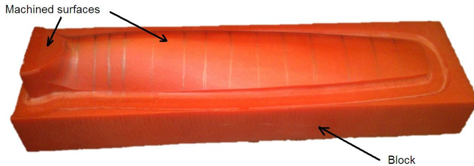
Figure 4. CAM manufactured freeform surfaces.
