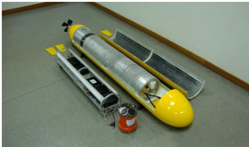
Figure 3. The Pirajuba AUV components. Inside the vehicle, it is shown the manoeuvre and the main vessels. On the left side, the inner platform of the main vessel, and the Doppler Velocity Log (DVL) sensor
