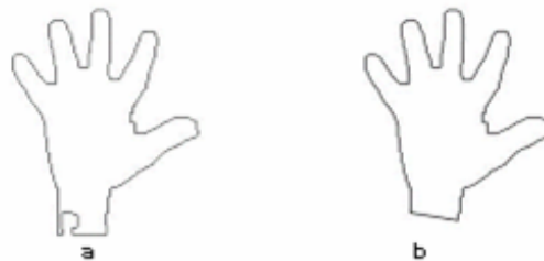
Figure 7. a) Hand boundary with the forearm. b) Hand boundary without the forearm.
