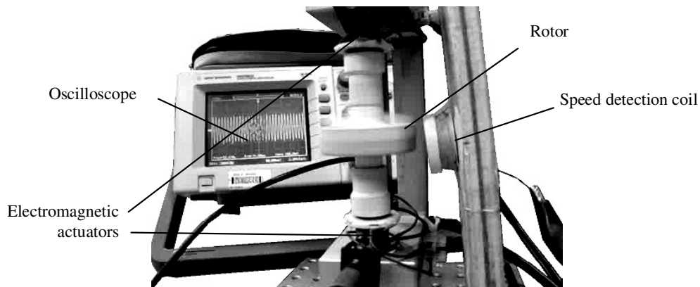
Figure 5. Set-up for testing the magnetic suspension.
