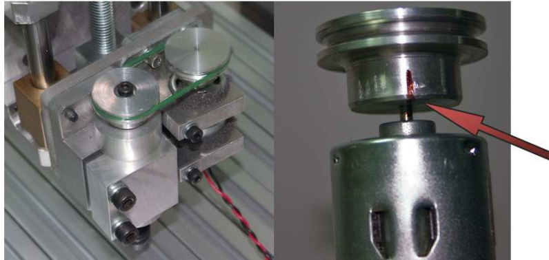
Figure 10. Marks made on shaft and pulley to check for slipping
