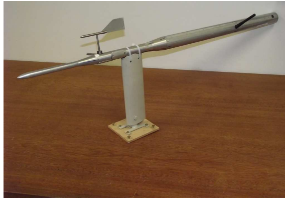
Figure 4. Final aspect of the Pitot tube
