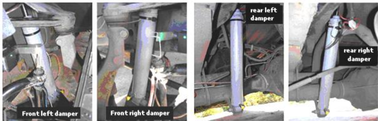
Figure 4. MR dampers prototypes installed in the pickup Ford Ranger.
