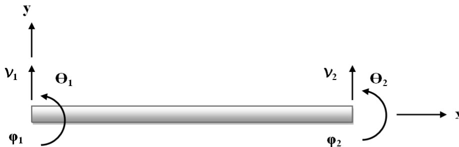
Figure 3: Beam finite element electromechanically coupled.
