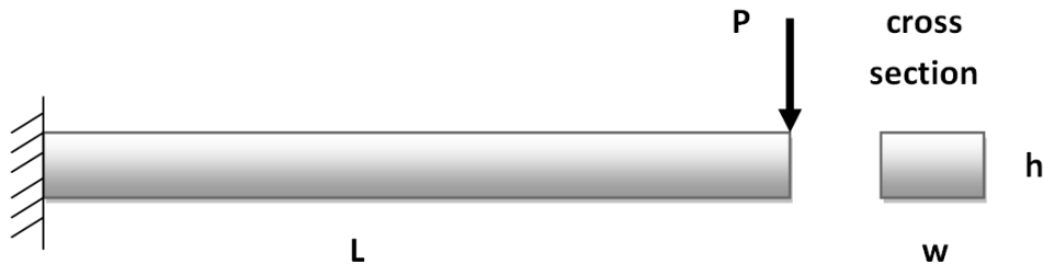
Figure 4: Beam model used in the simulation
