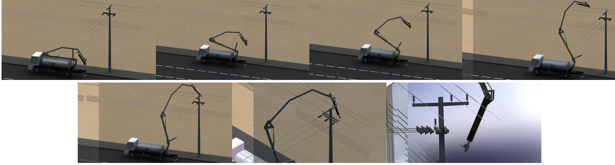
Figure 10. Sequence of the washing insulator operation.
