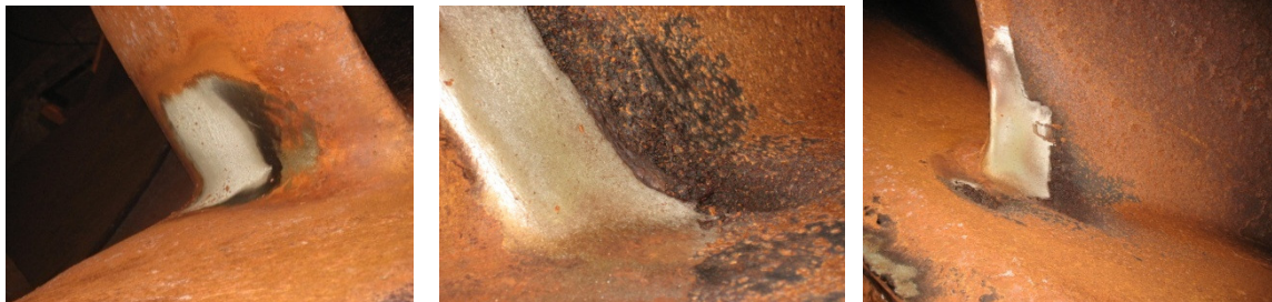
Figure 1- Hydraulic turbine blades damaged by cavitation.
