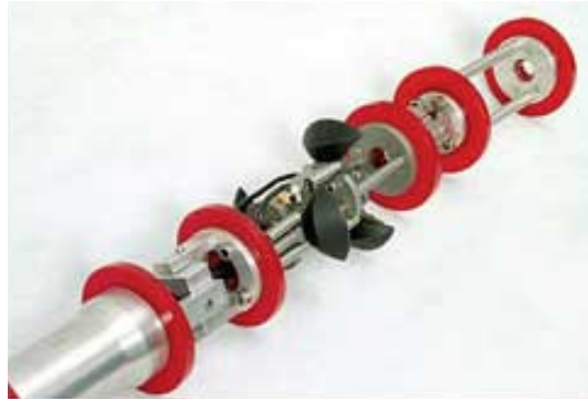
Figure 1. Pig with geometrical tool. (Da Silva,2001).
