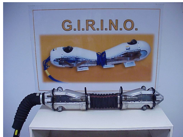
Figure 2. Prototype of G.I.R.I.N.O. traction module.
