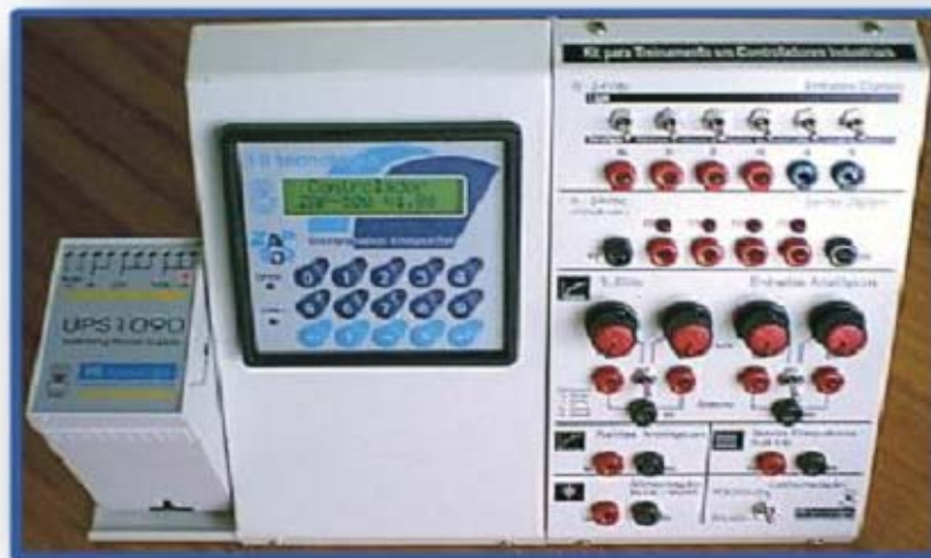
Figure 3. The ZAP500 PLC from Hitecnologia.
