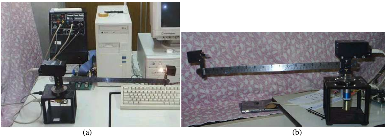
Figure 1. (a) The FLEXCAM Quanser System (b) Hub, camera and flexible beam
