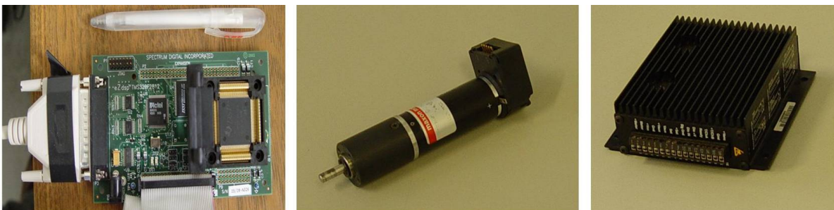
Figure 3. System devices, the DSP hardware, the DC motor, and the servo amplifier.
