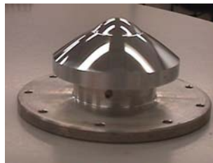
Figure 6. Hyperbolic mirror with two lobes
