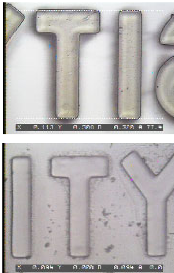
Figure 3: Good feature replication from SU-2075 master (top) to PDMS stamp (below). (100micron wide features)
