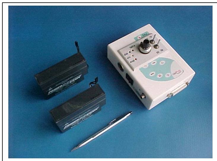
Figure 2. ATAH electronic controller unit (right side) and batteries (left side)
