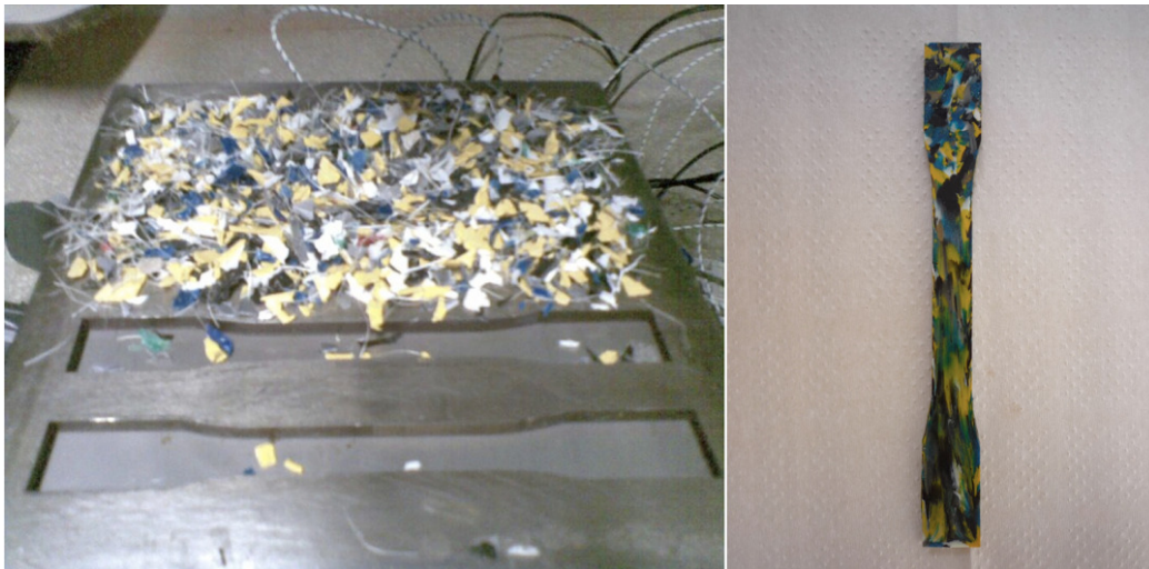
Figure 1 – Recycled HDPE tensile specimen mold and geometry.
