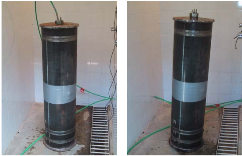
Figure 11 – 12" SCH 20 steel pipe with a repair of a hole of 10mm before and after testing
