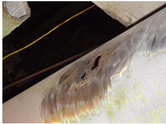
Figure 1 - Corrosion damage in produced water pipelines.
