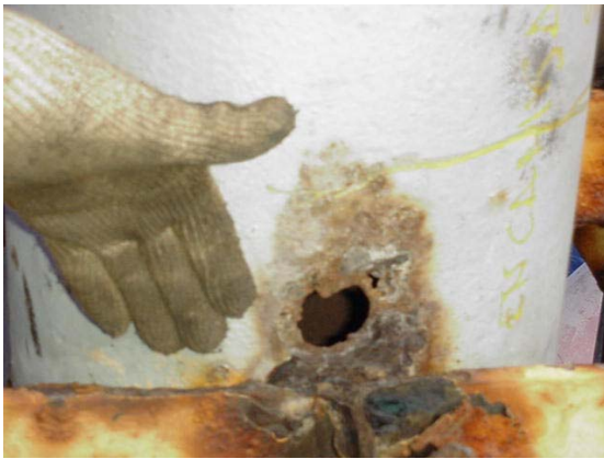
Figure 1 - Corrosion damage in produced water pipelines.
