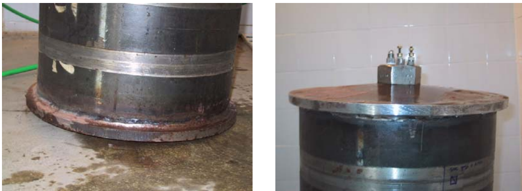
Figure 12 – Deformed caps after testing at 60 \text{ kg/cm}^2 and 80^\circ\text{C} .
