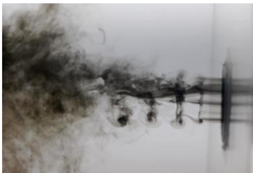
Figure 4. Flow visualized images of the free jet in Re \approx 11274 .
