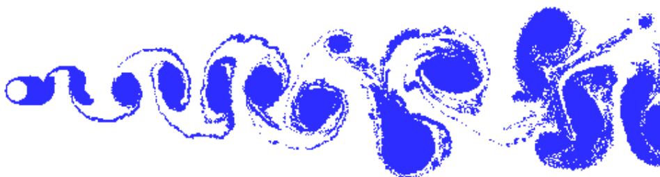
Figure 5. Vortex structure in the wake at t = 75.00 for an isolated circular cylinder ( Re = 1.0 \times 10^5 ).
