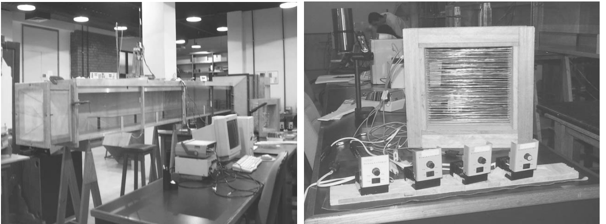
Figure 1. General view of the low-turbulence wind tunnel and the heating elements.
