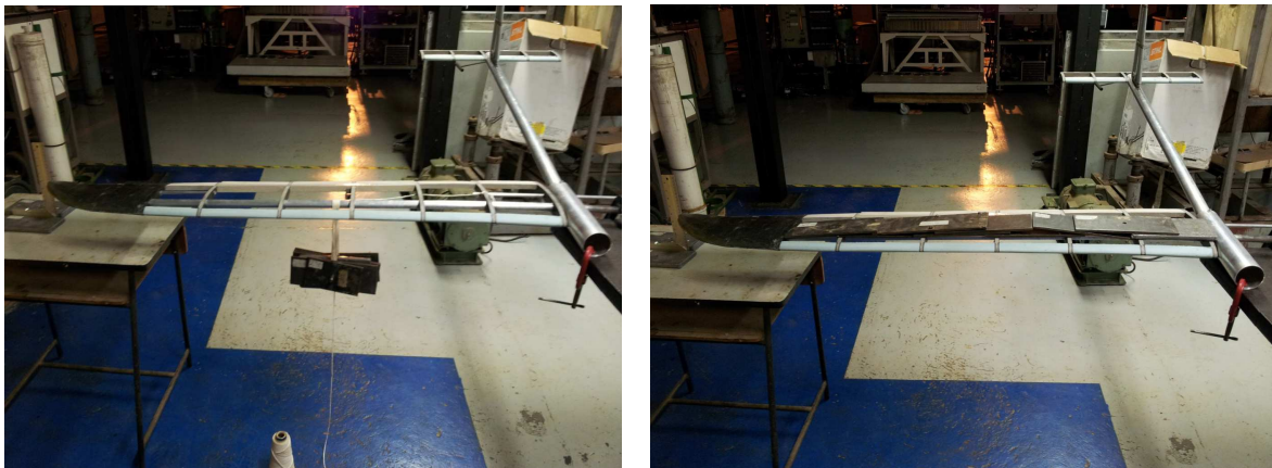
Figure 9. Experimental test with concentrated and distributed weight
