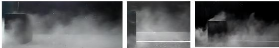
Figure 4. – Side view of the flow in near wake behind the cubic building.
