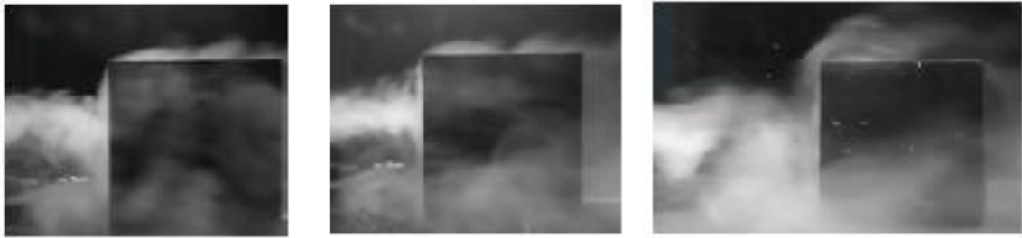
Figure 3. Side view of the incident flow around cubic building.
