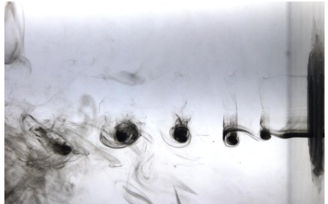
(b) Close view of the vortex shedding Re \approx 4000
