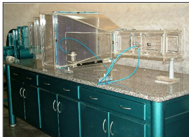
Figure 2. Aerodynamic tunnel of the Flow Visualization Laboratory (UNESP/FEIS).
