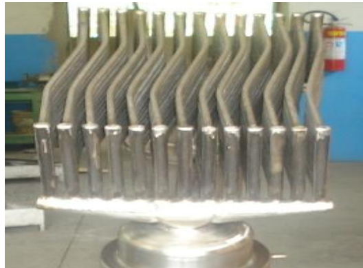
Figure 3. Hot heat exchanger
