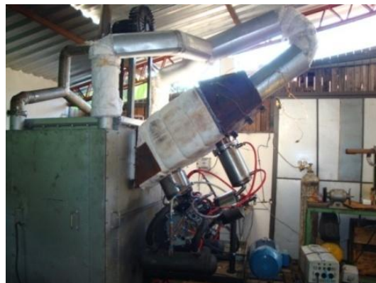
Figure 2. System of Stirling engine integrated with the biomass furnace
