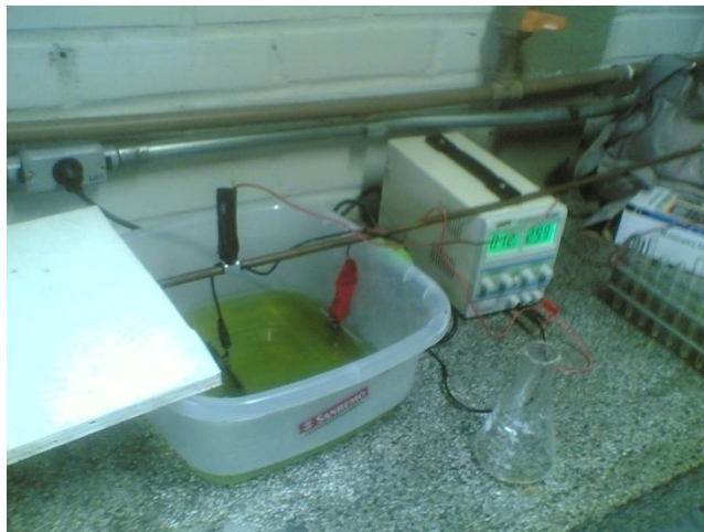
Figure 4. Electroflocculation cell for the separation of microalgae from an aqueous suspension.
