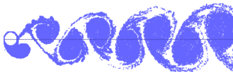
Figure 3 – Vortex cloud structure for transversely oscillating cylinder ( A_y/d=0.50 and f_{by}/f=1.0 ).
