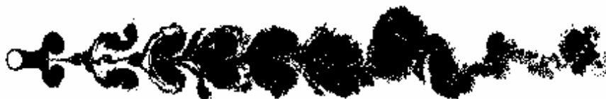
Figure 5. Symmetrical mode of vortex formation for in-line circular cylinder vibration ( A_x/d=0.5 and f_{bx}/f_{cd}=1.0 ).
