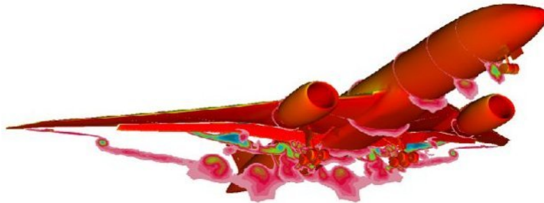
Figure 1. Numerical simulation over a commercial airplanes with the high-lift devices deployed.
