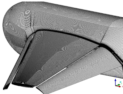
Figure 4. Surface mesh for configuration one (hexahedral mesh) .
