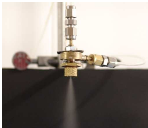
Figure 3. Photo of a leaking test of the blurry injector.
