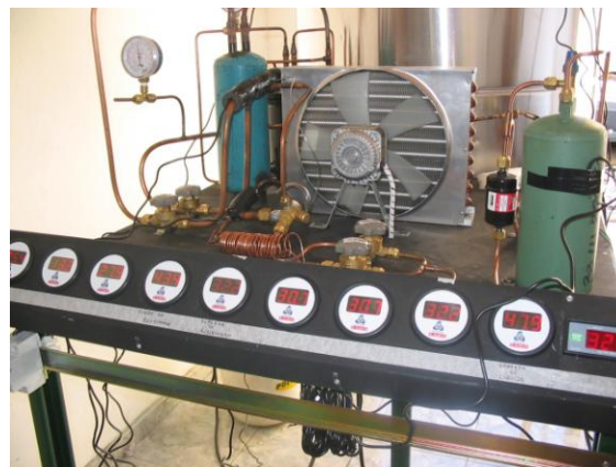
Figure 5: Overview of Heat Pump Source: Silva, IC-refrigeration laboratory - UFMG [20]
