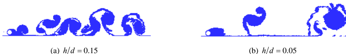
Figure 5. Position of the vortices in the wake at the end of the simulation of a circular cylinder in ground effect
