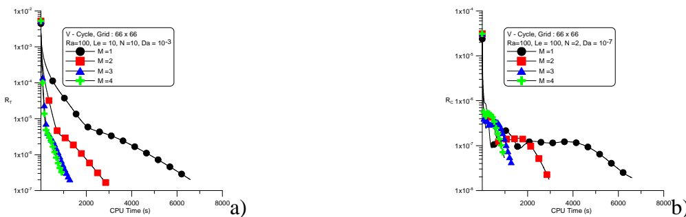
Figure 5 - Residue history for square filled with porous material Ra = 100 , Le = 100 , Da = 10^{-7} , N=2 , V-Cycle: a) Temperature; b) Mass concentration
