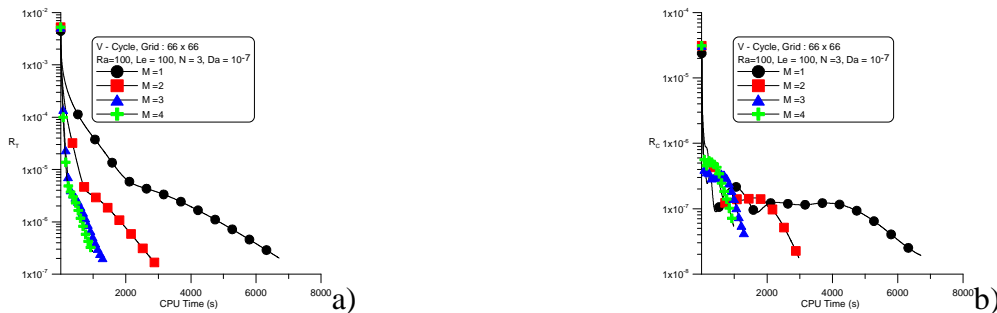
Figure 6 - Residue history for square filled with porous material Ra = 100 , Le = 100 , Da = 10^{-7} , N=3 , V-Cycle: a) Temperature; b) Mass concentration
