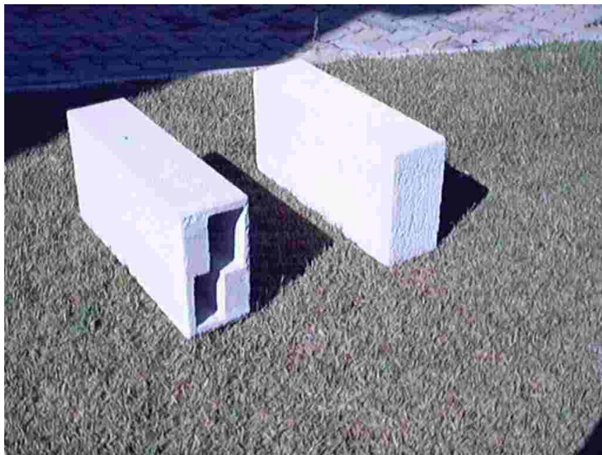
Figure 11. Prototype and original concrete brick.
