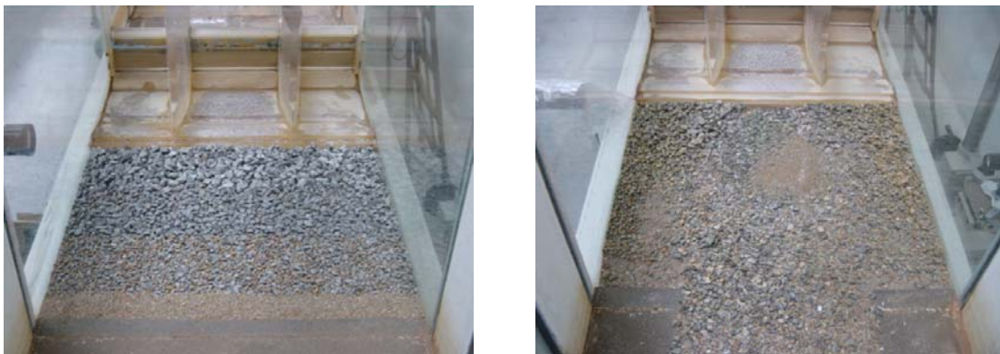
Figure 9: Illustration of the rock protection bed and the observed scour hole.
