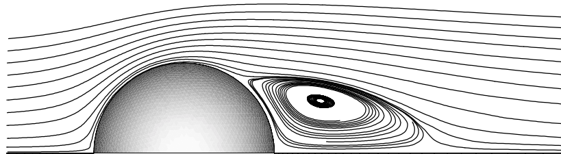
Figure 8 – Viscous incompressible flow around a sphere: streamlines.
