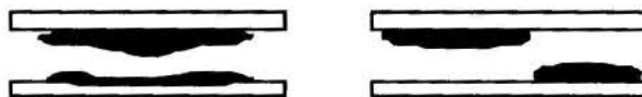
Fig 2a - Typical separation for steel plates. Both sides are heavily fouled, and the fracture occurs inside the oil drop. It is very hard to clean both surfaces.
