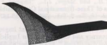
Figure 3: View of a typical 3-D computational grid.
