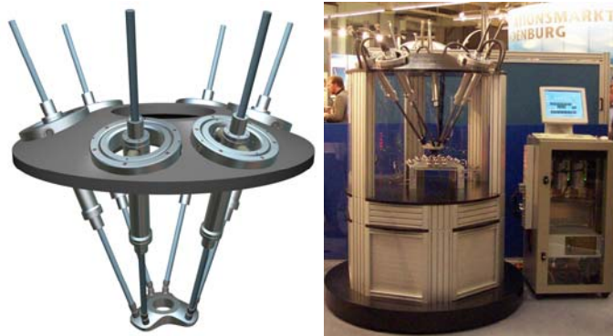
Figure 2 – Hexapod PaLiDa: MBS model and test bed.
