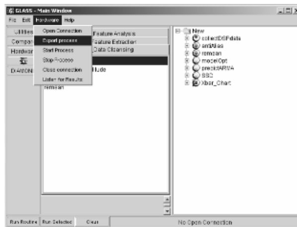
Figure 2. - Screen shot capturing the added Hardware drop down menu. The menu items displayed correspond to commands that can be sent to the node. Notice that confirmation or errors of the commands sent are displayed in the process bar at the bottom.
