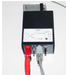
Figure 4. Picture of the Low Cost Impedance Measurements (LCIM) equipment.
